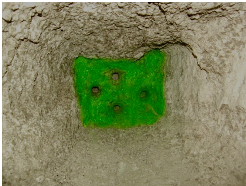
Figure 4.9. Typical Extended Relief Round (The resulting profile from Test 17 shows the bootleg left from each of the four extended relief holes. The back face of the cut has been painted green to accentuate its profile.)
